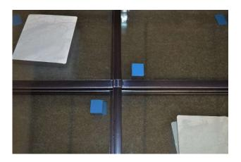
Toughened glass may show visual distortions which are accentuated by reflections in sealed units. This is a natural phenomenon and not a fault.
